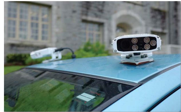
Digital Chalking using Licence Plate Recognition Technology
